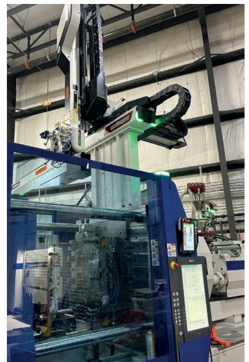
The injection molding machines in the plant are equipped with WITTMANN linear robots.
