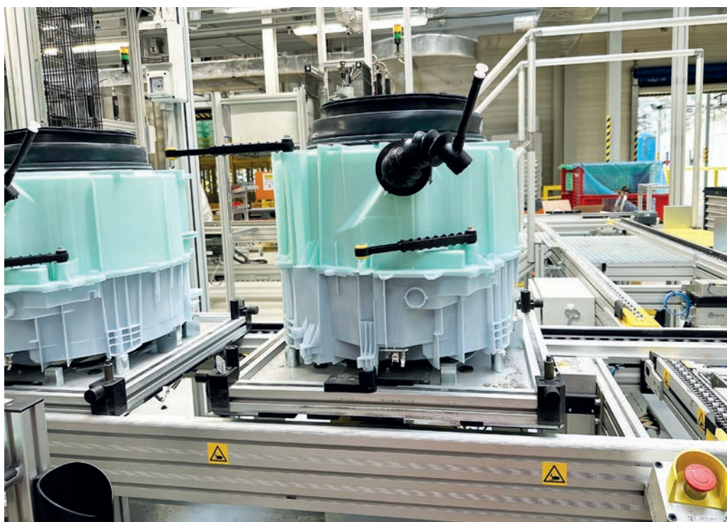
The light green and gray housing halves are welded together to enclose the washing drum inside the finished washing machine. Most recently, BSH in Poland produces both of these injection-molded parts in its own injection molding shop.
