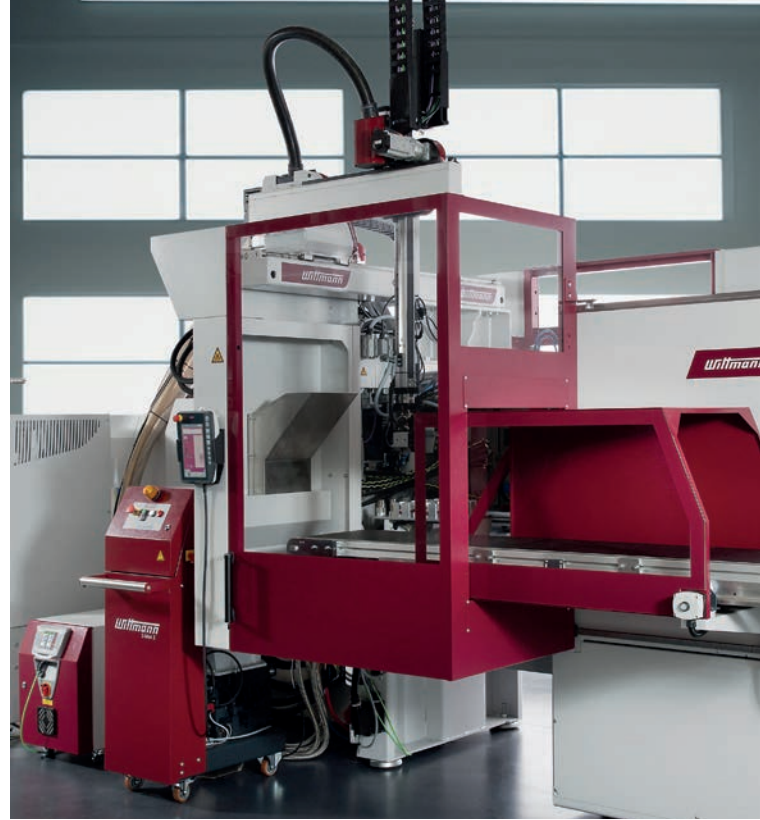
Designed as an Ingrinder production cell, the in-line recycling system requires hardly any additional space. The sprue need not leave the protective housing of the machine to be transferred to the granulator.
