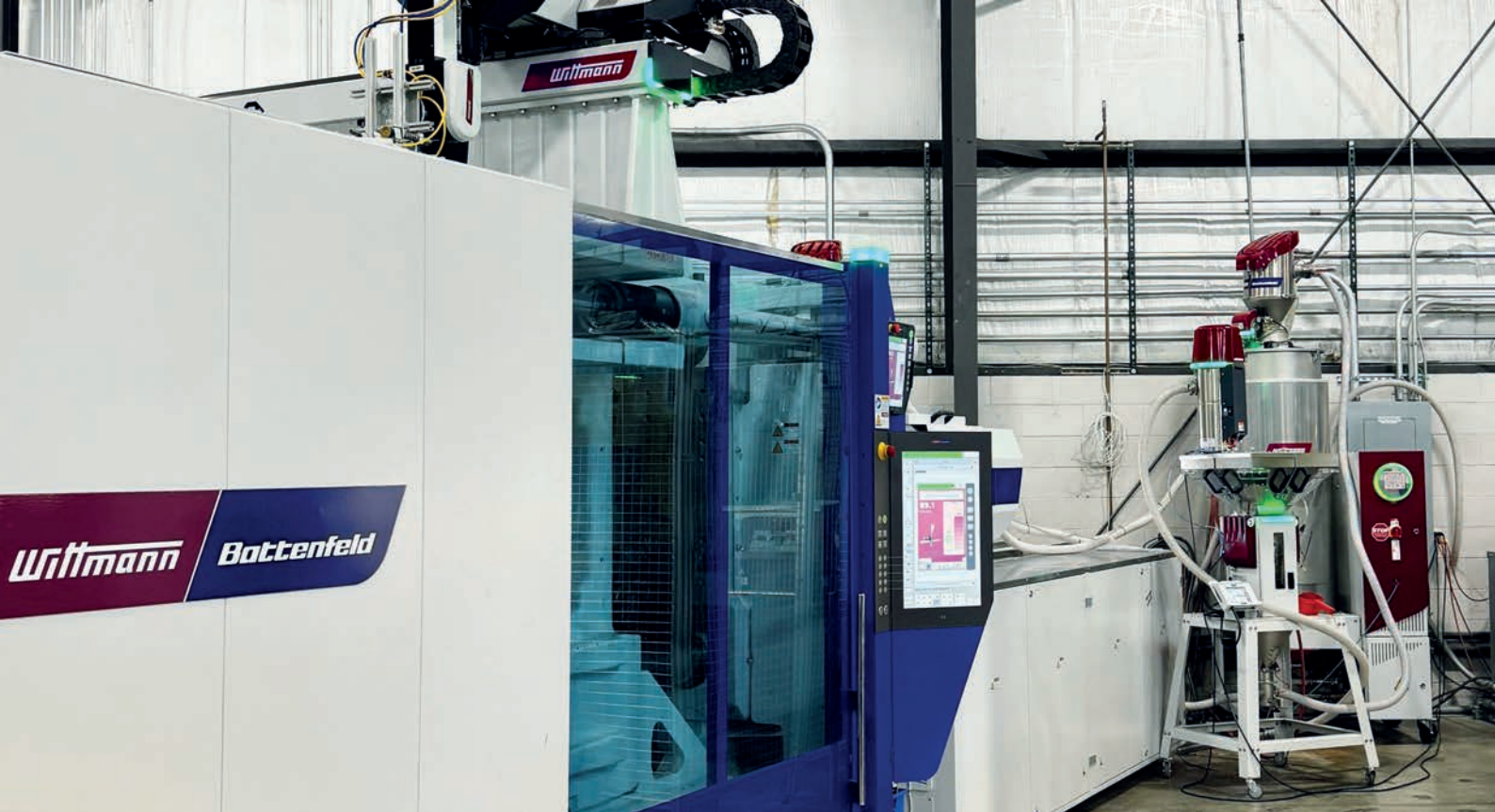
The Gravimax dosing units help with color management. They communicate directly with the injection molding machine and all other components of the production cell via Wittmann 4.0.
