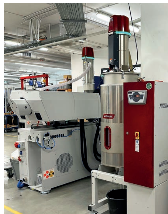
PETG places special demands on the drying process. The WITTMANN team has modified the Drymax dryers accordingly for their customer Bell.
