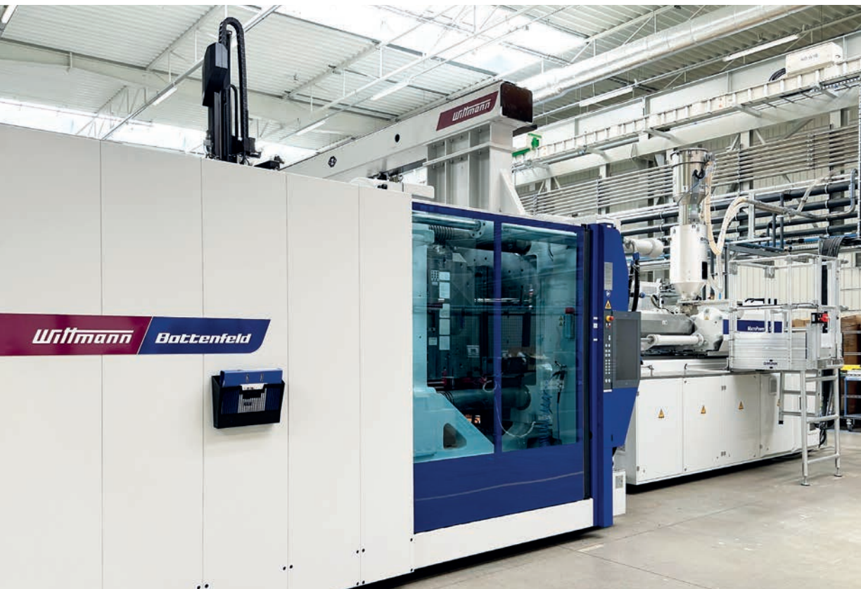
At the BSH plant in Łódź, all MacroPower injection molding machines are equipped with W863 pro linear robots.
