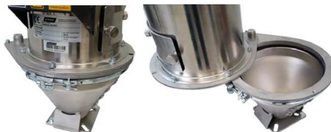
*The pivoting device for the machine hopper can be retrofitted*
