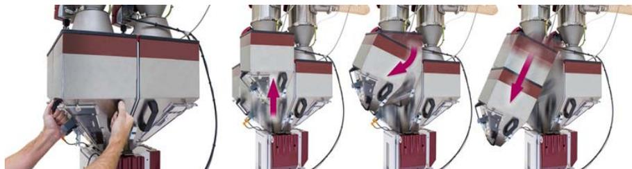
***Push the hopper upwards, unscrew it and take it off;
