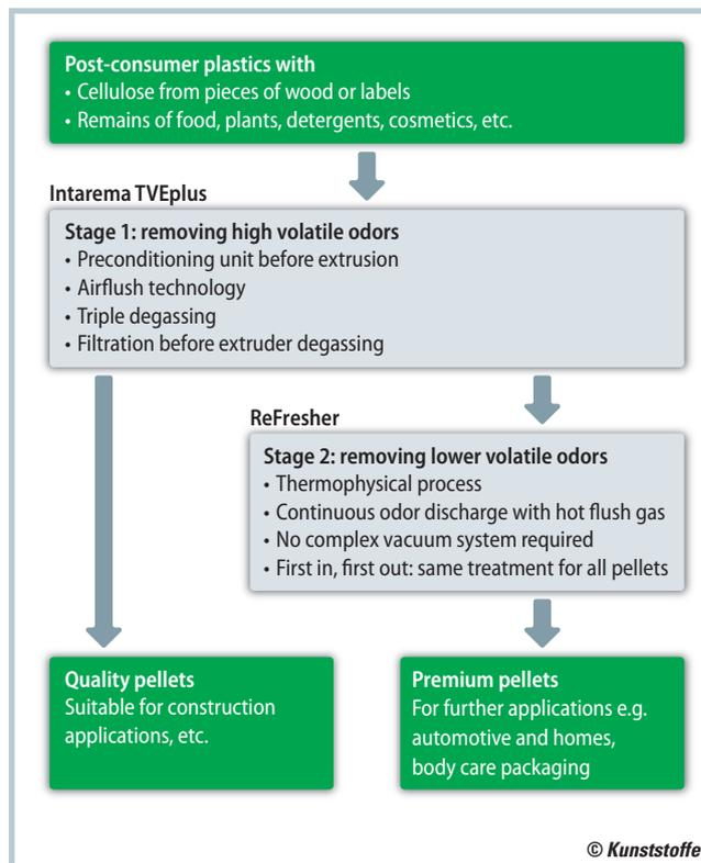
**Fig. 1.** Process overview: Odor-reduced pellets are created when not only the low molecular but also the low volatile, high molecular substances are removed (source: Erema)
