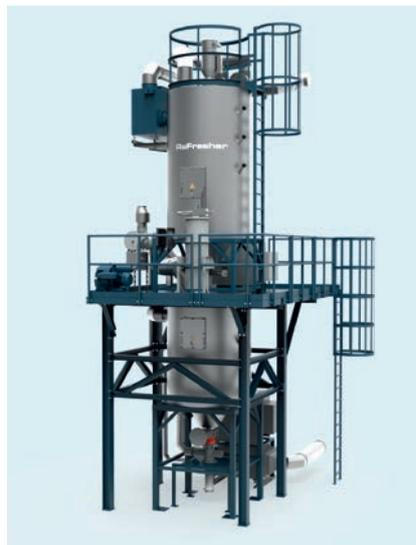
**Fig. 4.** To remove the odors of low volatile, high molecular substances the ReFresher uses the energy of the pellets which have been preheated through extrusion. A hot stream of purge gas ensures continuous odor discharge – depending on the application with a dwell time of between 7 and 32 hours. The dwell time itself is kept the same for all pellets through design measures (“first in, first out”)
