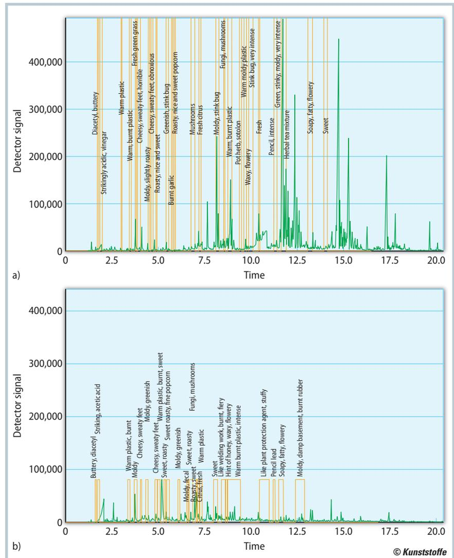
**Fig. 2.** VOC values (green) and odor perception (orange): a) Assessors can identify odors even if the odor-causing substances (VOCs) are below the detection threshold, i.e. no longer registered by conventional detectors and no peak is visible on the chromatogram; b) lower VOC concentrations correlate with lower odor perception (source: TU Graz)
