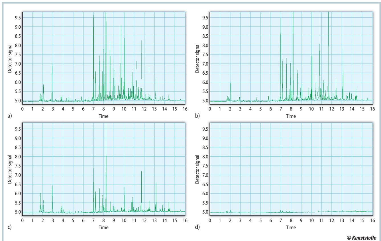
**Fig. 3.** Gas chromatography VOC analysis to assess odor optimization: The height and width of a peak are an indicator of the amount of the substance. a) Input material before extrusion process, b) after the preconditioning unit (before entering the extruder), c) after the extrusion process with Intarema TVEplus RegrindPro, d) after a further 7h dwell time in the ReFresher (source: Fraunhofer IVW)
