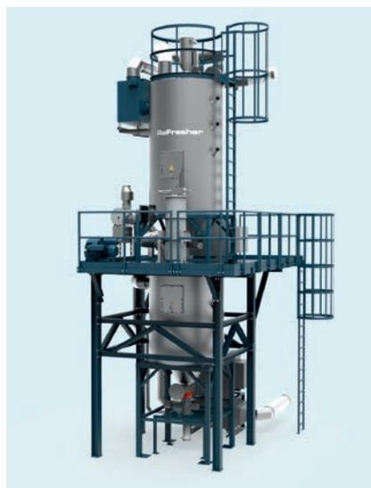
**Fig. 4.** To remove the odors of low volatile, high molecular substances the ReFresher uses the energy of the pellets which have been preheated through extrusion. A hot stream of purge gas ensures continuous odor discharge – depending on the application with a dwell time of between 7 and 32 hours. The dwell time itself is kept the same for all pellets through design measures (“first in, first out”) (© Erema)
