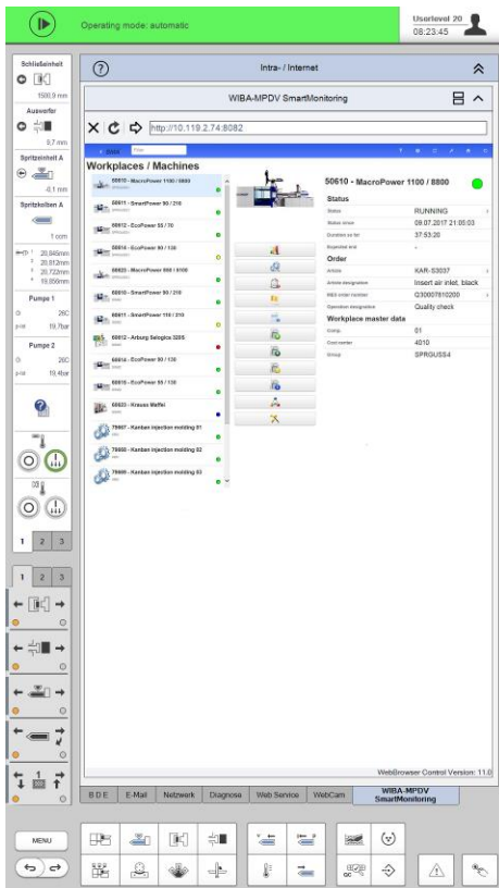
Fig. 7: Integration of the WIBA-MPDV SmartMonitoring module in the UNILOG B8 control system (Courtesy of: WIBA, MPDV Mikrolab GmbH)
