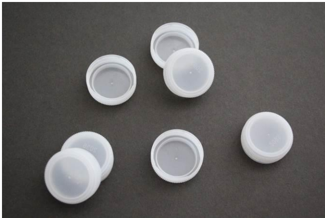
Fig. 2: Closing caps made of HDPE – manufactured on the EcoPower Xpress
