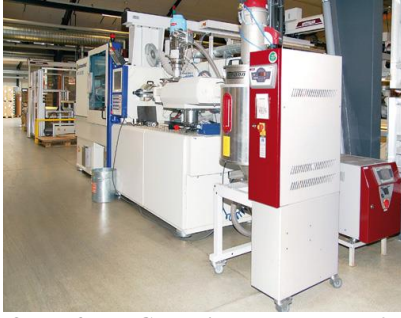
One of HN Group's new TEMPRO plus D180 high temperature water controllers (right, in the background), connected to a WITTMANN BATTENFELD injection molding machine. This production cell also comprises a WITTMANN CNC robot on the machine and a WITTMANN material dryer (in the foreground).
