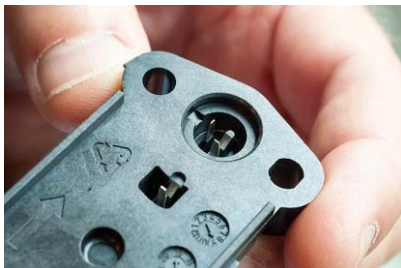
Insert-molded part, produced at the HN Group's plant in Billund, Denmark.
