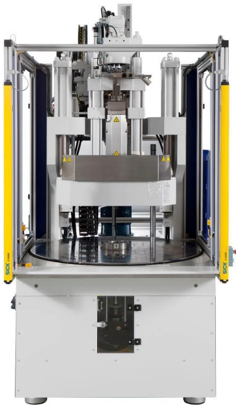
Fig. 4: CM R 40 vertical injection molding machine – freely accessible from all sides
