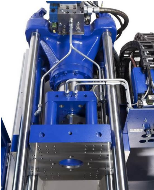
Fig. 3: Central hydraulic clamping unit of the SmartPower
