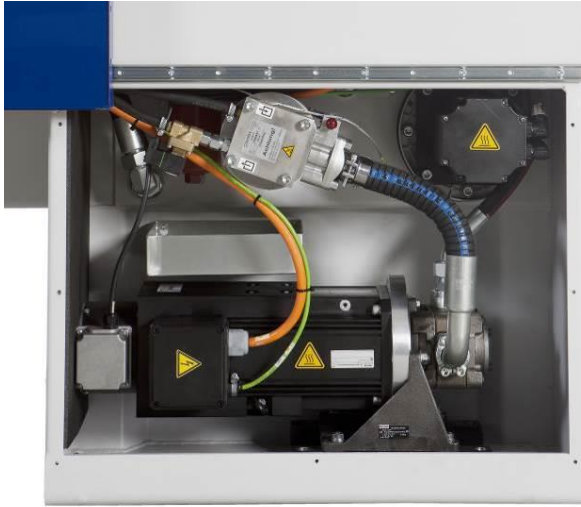
Fig. 2: Highly dynamic servo motor of the SmartPower
