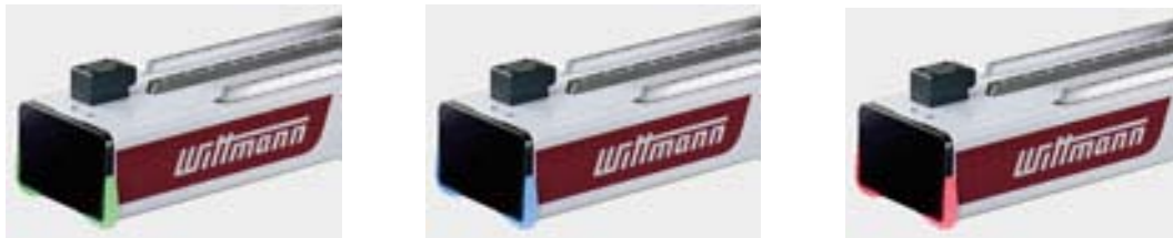
The ambiLED signal lamp shows different operational states Green light: the robot is working automatically Blue light: manual intervention required Red light: safety gate is open
